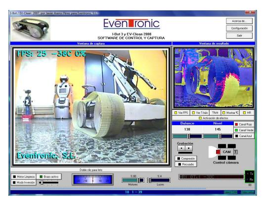
Image capture of Eventronic control program. Optionally you can read the temperature and humidity inside the ducts and show (with video overlay) on the screen.
